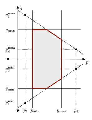
Figure 6-6: Generator P-Q Capability Curve
