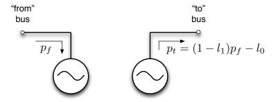
Figure 7-3: Equivalent "Dummy" Generators
