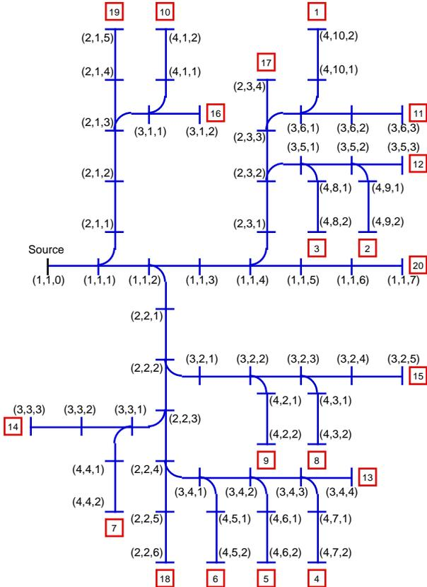
**Figure 1** Example of Bus & Lateral Indexing
